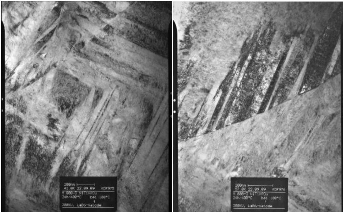
Figure 5.15: TEM micrographs of \text{Ni}_{45.3}\text{Cu}_5\text{Ti}_{29.7}\text{Hf}_{20} aged for 24hours at 400^\circ\text{C}
