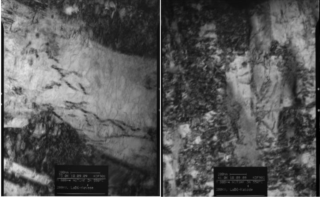
Figure 5.16: TEM micrographs of \text{Ni}_{45.3}\text{Cu}_5\text{Ti}_{29.7}\text{Hf}_{20} aged for 3 hours at 550^\circ\text{C}
