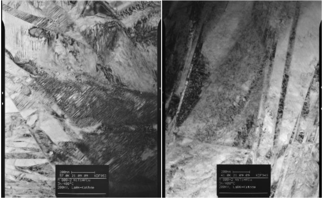
Figure 5.14: TEM micrographs of \text{Ni}_{45.3}\text{Cu}_5\text{Ti}_{29.7}\text{Hf}_{20} aged for 3hours at 400^\circ\text{C}
